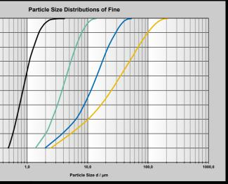
Extensive and detailed testing with the new NEA GRC classifier revealed a particularly high cut efficiency as well as excellent yields and throughputs. The diagram shows different particle size distributions of the fine material fraction.
