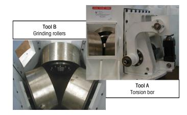
Grinding by contact of the rollers with turntable
