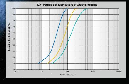
The diagram shows different particle size distributions of the fine material fraction
