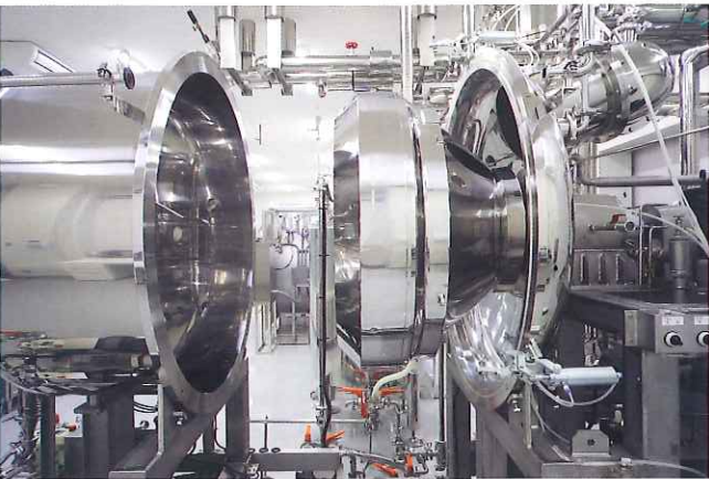
Spinning cone housing can be easily open in order to facilitate inspection and cleaning
